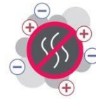
Odorous gases and aerosols oxidize on contact with oxygen ions and are neutralized
